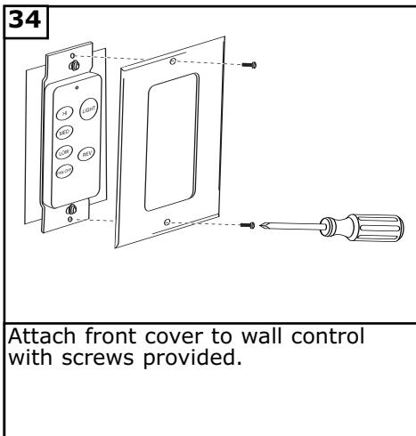
34 Attach front cover to wall control with screws provided.
